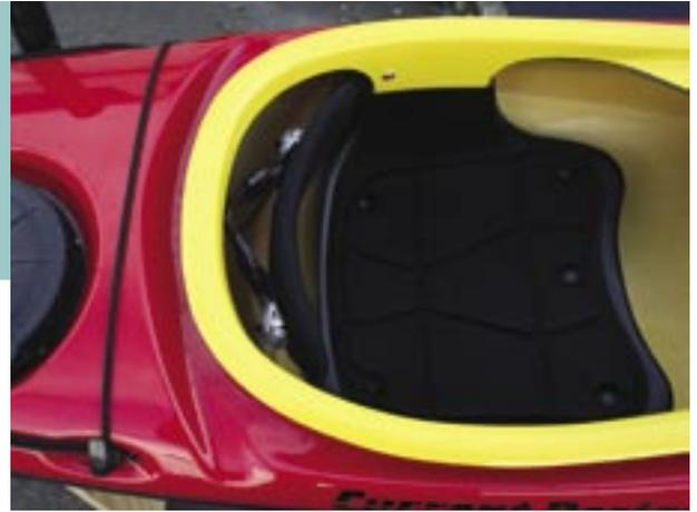
The back band is well supported by bungees and is adjusted with a pair of ratcheting buckles.
